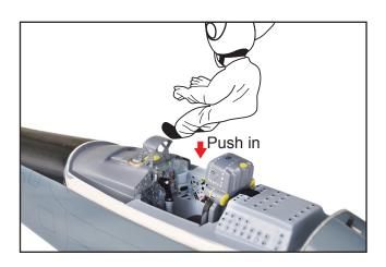
Use glue to secure the canopy to the fuselage. The shape of the canopy, so make sure to install it in the correct direction.
