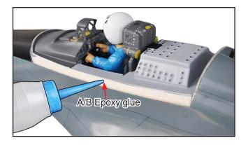
Position the canopy so the rear frame on the canopy is aligned with the rear edge of the cockpit opening. Use canopy glue to secure the canopy to the canopy hatch. Use low-tack tape to hold the canopy in position until the glue fully cures. Wrap the tape completely around the canopy hatch, as the tape does not stick well to the covering. We used balsa sticks to hold the lower edges of the canopy tightly against the canopy hatch.
