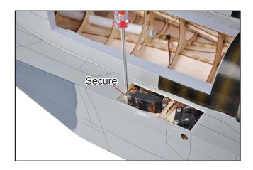
Repeat the procedure to install the second elevator servo in the opposite servo tray.
