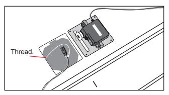
□ 4) Place the servo into the servo tray. Center the servo within the tray and drill 1.5mm pilot holes through the block of wood for each of the four mounting screws provided with the servo.
