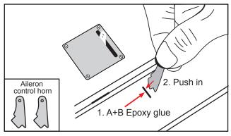
$\Box$  3) Repeat the procedure to install the control horn on the opposite aileron.
