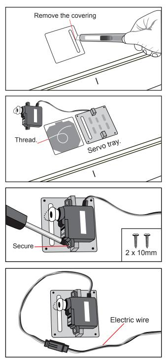
□ 3) Using the thread as a guide and using masking tape, tape the servo lead to the end of the thread: carefully pull the thread out. When you have pulled the servo lead out, remove the masking tape and the servo lead from the thread.
