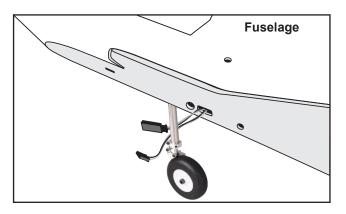
□ 1) Attach the aluminium tube into the fuselage.
